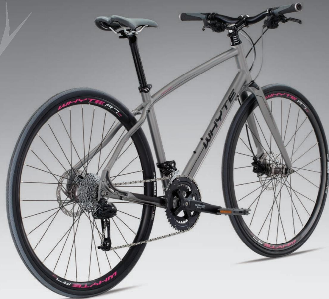
Lightweight aluminium frame with compact geometry / Carbon fibre fork with alloy steerer tube / SRAM 2x10spd compact gearing / Tektro hydraulic disc brakes
