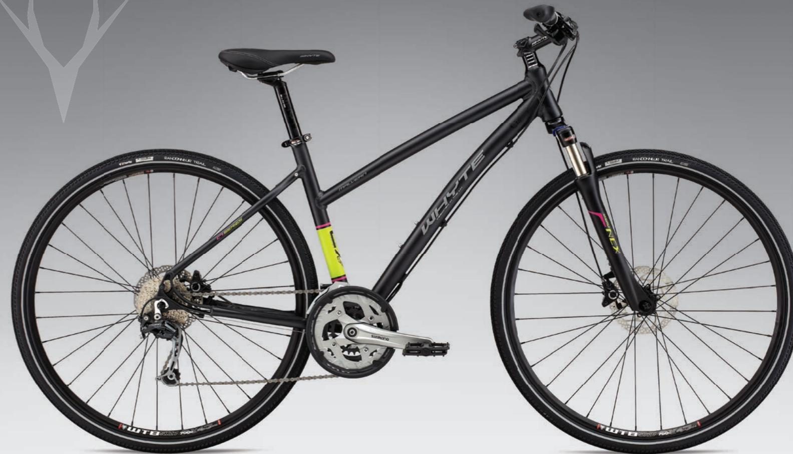
SR Suntour suspension with Hydro lockout is lightweight thanks to an alloy steerer tube / Powerful Shimano disc brakes / Lightweight aluminium frame with partially dropped top tube
