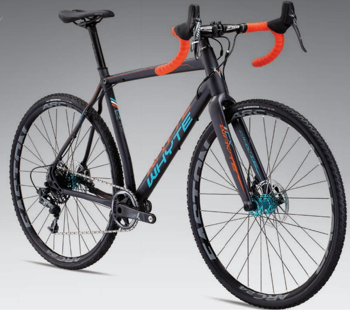
SRAM Force 1 1x11spd drivetrain and hydraulic disc brakes / Easton ARC-24 tubeless rims with Maxxis TR tyres / Whyte CX carbon disc fork with 15mm Axle and internal cable routing
