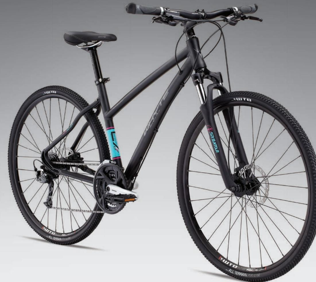
SR Suntour suspension fork with Hydro lockout / Partially dropped top tube is stronger than a fully dropped frame / Shimano 3x9spd gearing / Tektro hydraulic disc brakes
