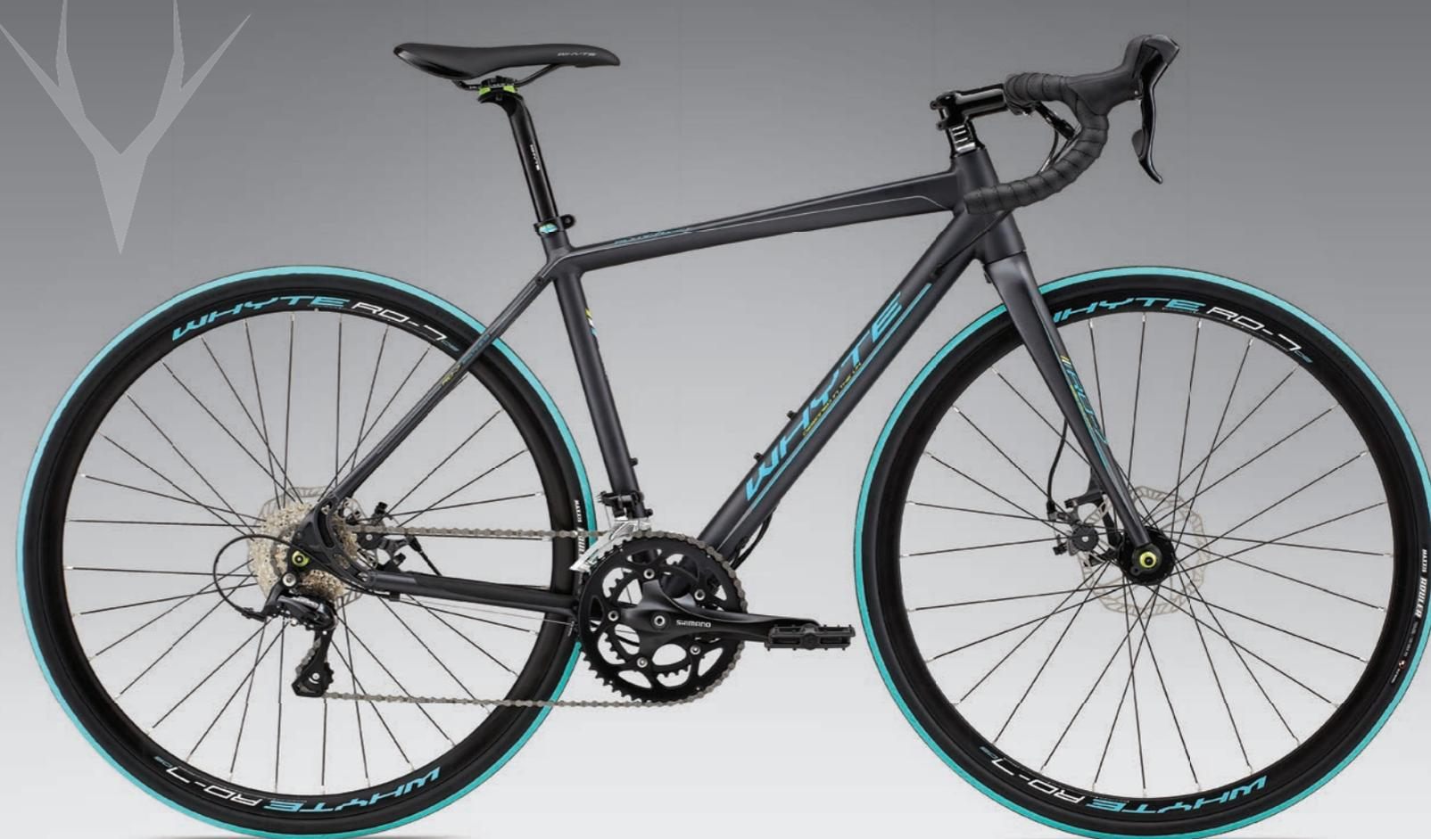
Lightweight disc-specific aluminium frame with alloy fork / Shimano 9spd compact gearing with wide range rear cassette / Powerful mechanical disc brakes / Internal fork routing
