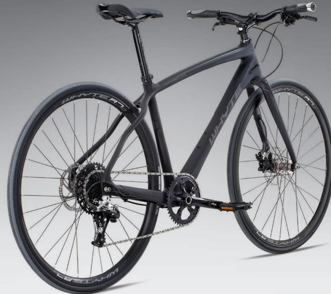
Full carbon frame is 300g lighter than aluminium / SRAM Rival 1, 11 by 11 groupset/ lightweight carbon fibre fork with internal cable routing
