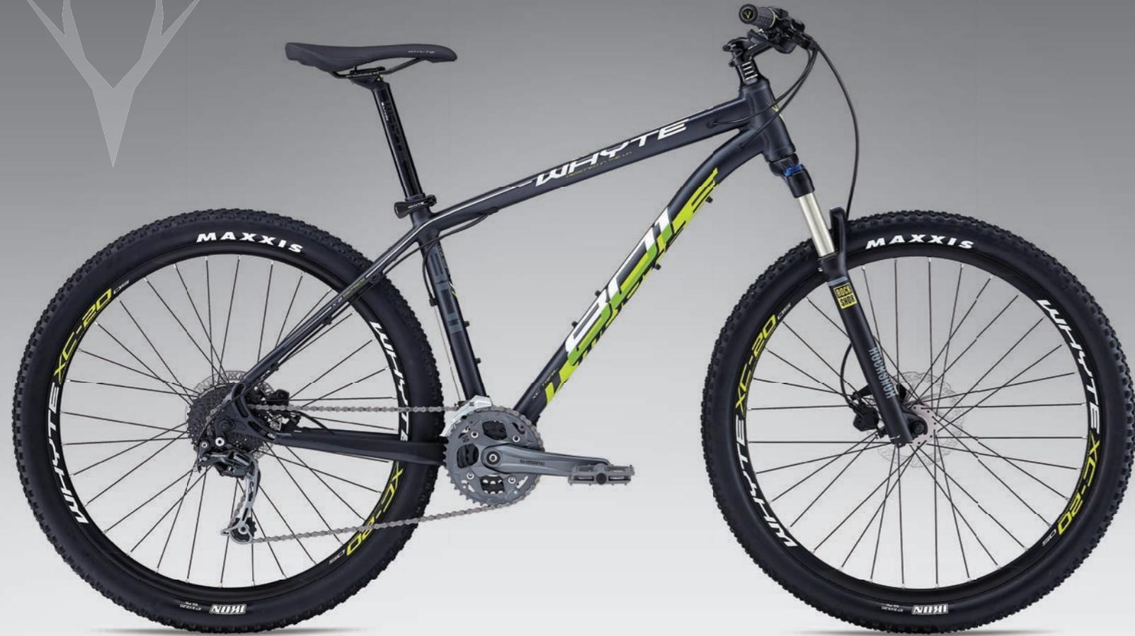
Shimano 3x9spd drivetrain provides gears for all terrain / Maxxis Ikon tyres roll fast and grip well / RockShox 30 Silver fork with TurnKey lockout and Solo Air
