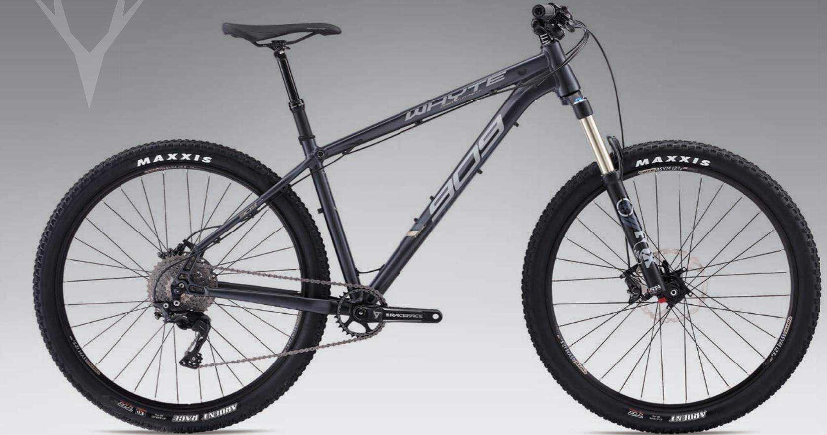
Shimano's new 1x11 XT M8000 combined with RaceFace Clinch chaining and BB30 axle / UK-made Hope Evo rear hub / Fox 34 Performance fork with FIT4 Damper
