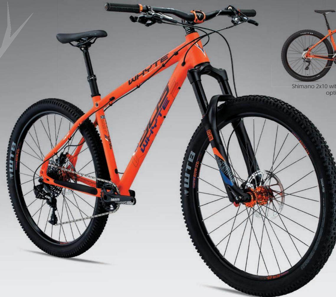
SRAM GX, 1x11 RockShox Yari RC fork / Internally routed KS CRUXI Dropper Post / Whyte custom 760mm bar and short gravity stem/ WTB front and rear specific TCS tyres and rims
