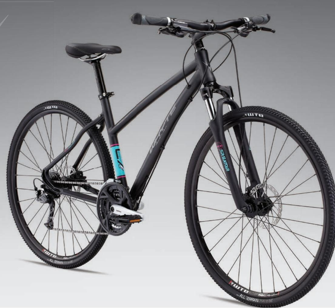
Wide-ratio 3x10spd Shimano Deore/LX gearing / Lightweight aluminium frame with partially dropped top tube / Vittoria Randonneur Trail tyres with double puncture protection
