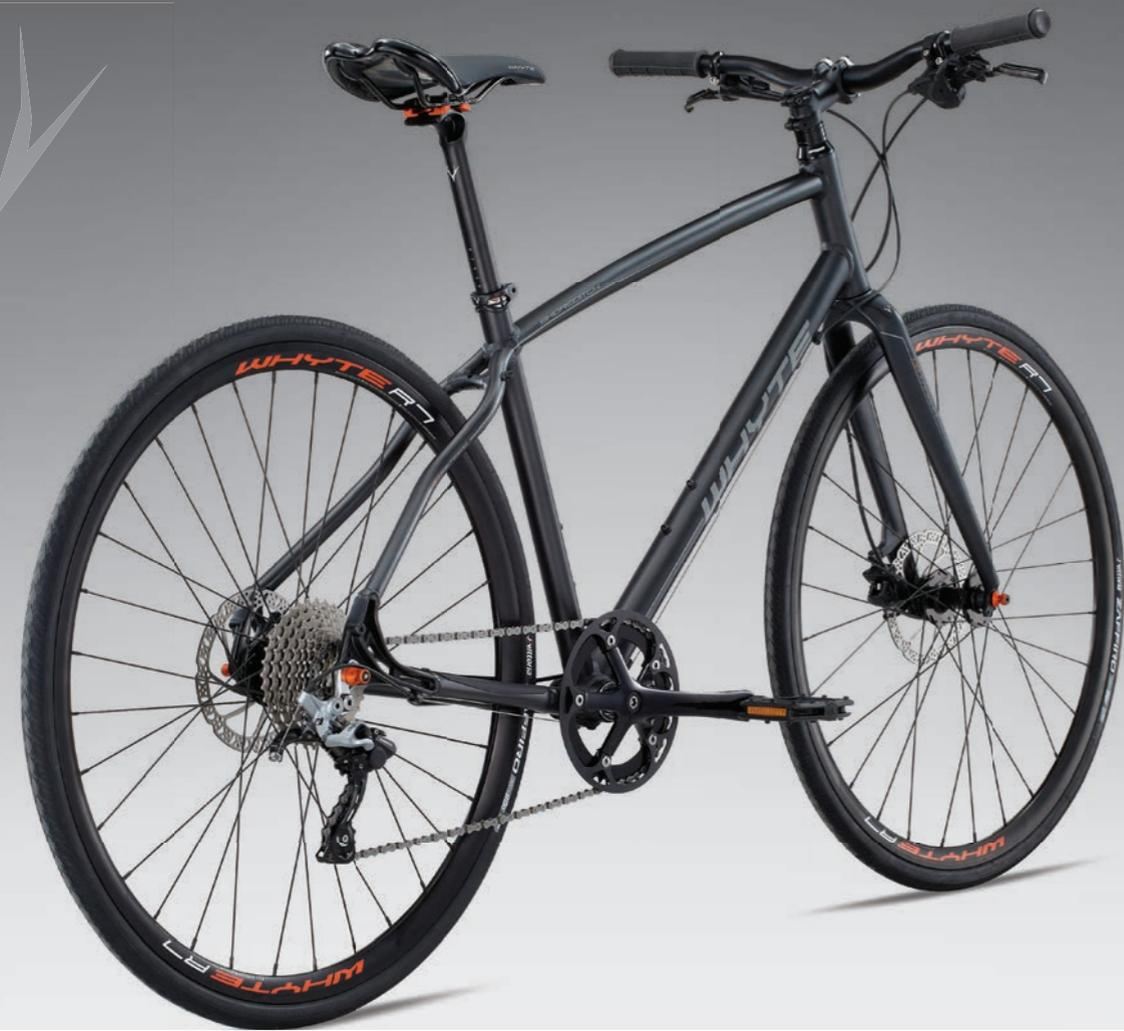
Lightweight aluminium frame / 1x10spd Shimano mountain bike gearing for city-proof performance / Reliable and powerful Tektro hydraulic disc brakes
