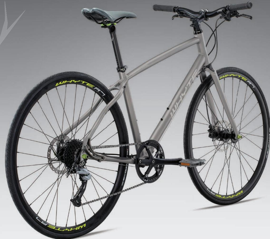
Tektro hydraulic disc brakes / 1x9spd Shimano drivetrain for urban simplicity / Lightweight aluminium frame
