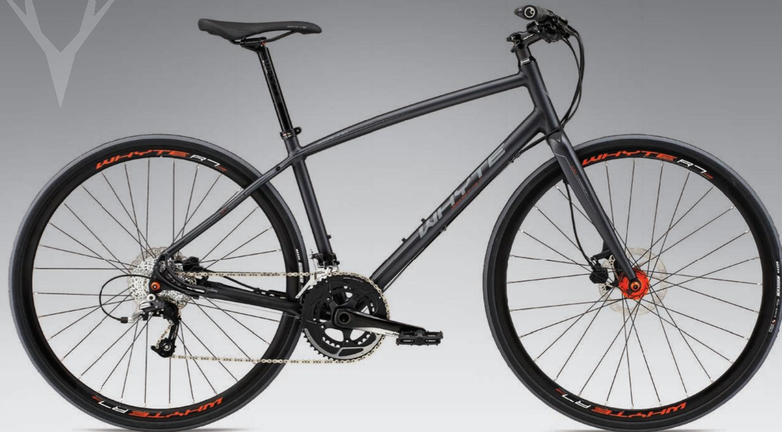
SRAM Rival 22 groupset / lightweight aluminium frame and carbon fibre fork / Powerful Tektro Gemini hydraulic disc brakes
