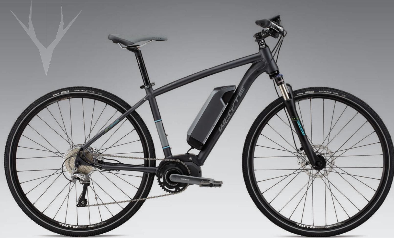
Shimano STEPS e-Bike drive and control unit/SLX gearing / Shimano Disk Brakes / Vittoria Randonneur Trail tyres with double puncture protection
