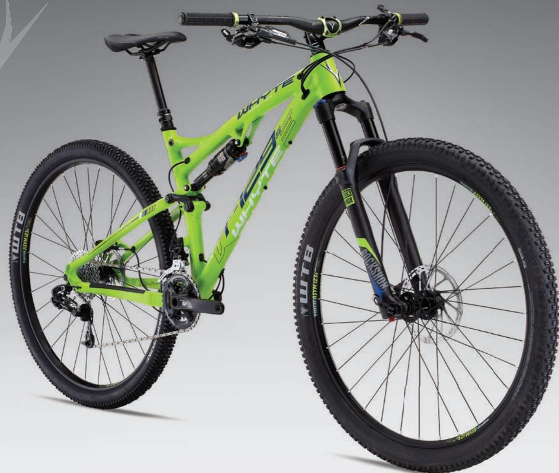
RockShox Reverb Stealth seatpost, Revelation RL fork and Monarch DebonAir shock / SRAM GX 2x10spd drivetrain/ WTB tubeless-ready offset rims and tyres
