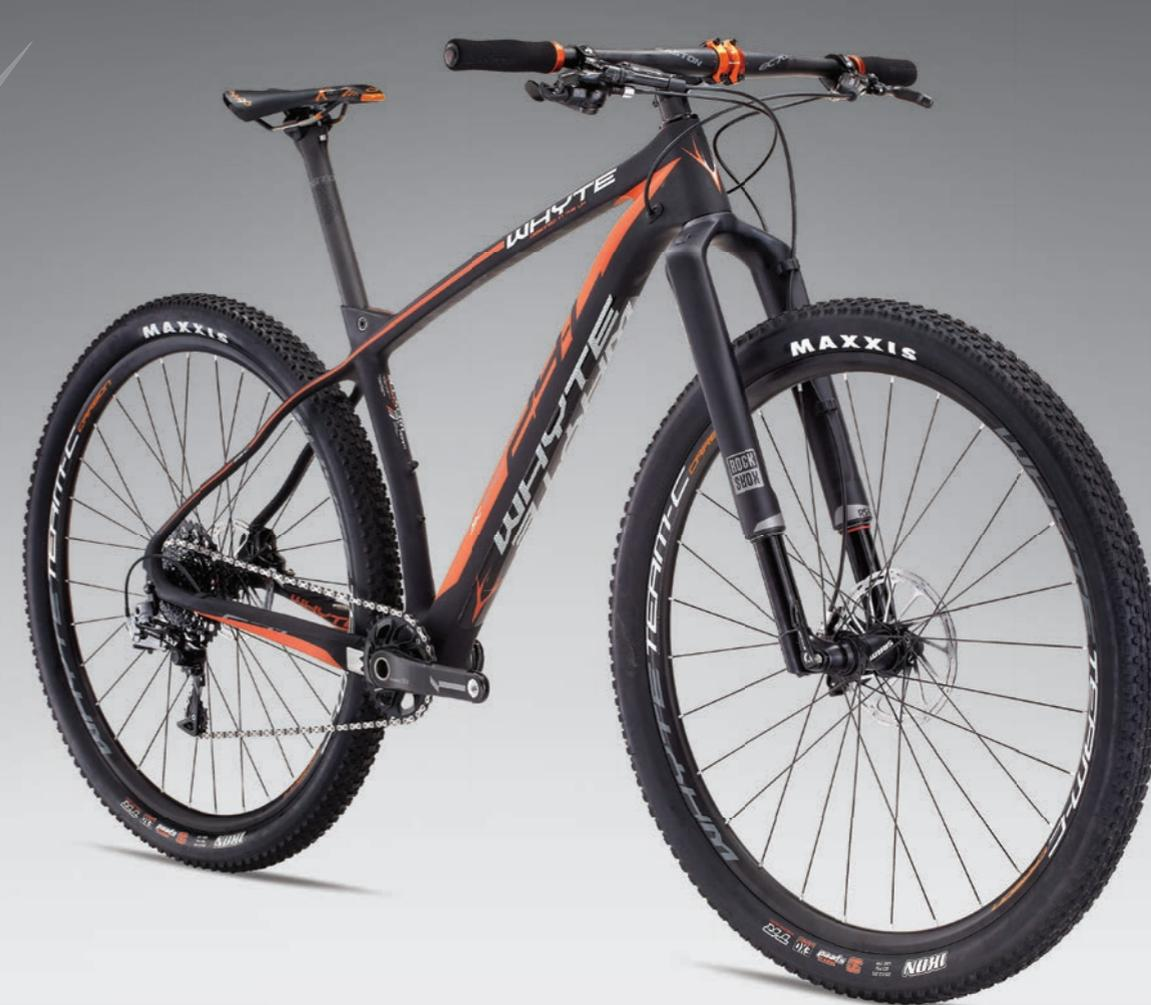
RockShox RS1 inverted XC fork / SRAM XX1 1x11spd drivetrain / SRAM Guide RSC brakes / Easton EC-70 seat post and 720mm handlebar / Intergrip
