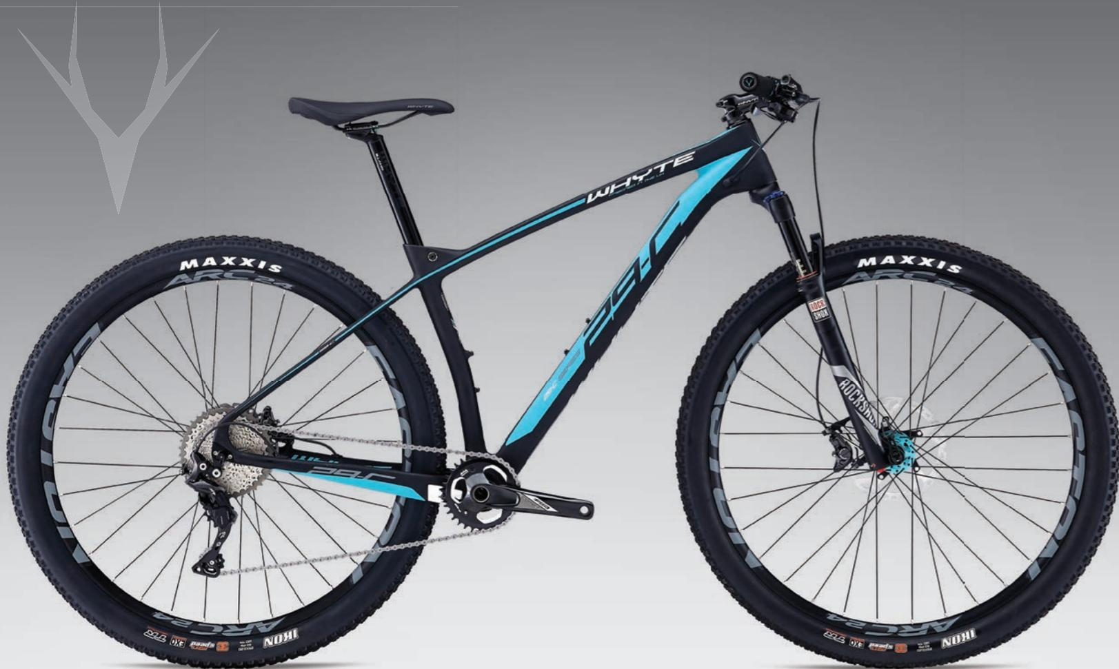
Light and stiff Easton/DT/Whyte Wheelset / Shimano XT brakes and 1 by 11 drivetrain / RockShox Reba RL fork with 15mm Maxle Lite / Intergrip
