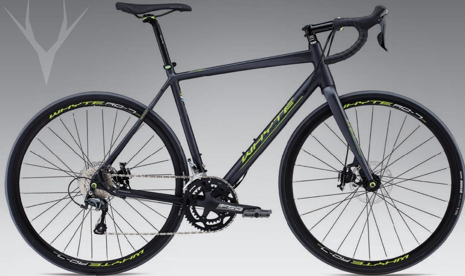
Disc-specific aluminium frame with carbon fibre fork / TRP HyRd mechanical/hydraulic disc brakes / Shimano Tiagra 10spd compact gearing with wide range rear cassette / Internal fork routing
