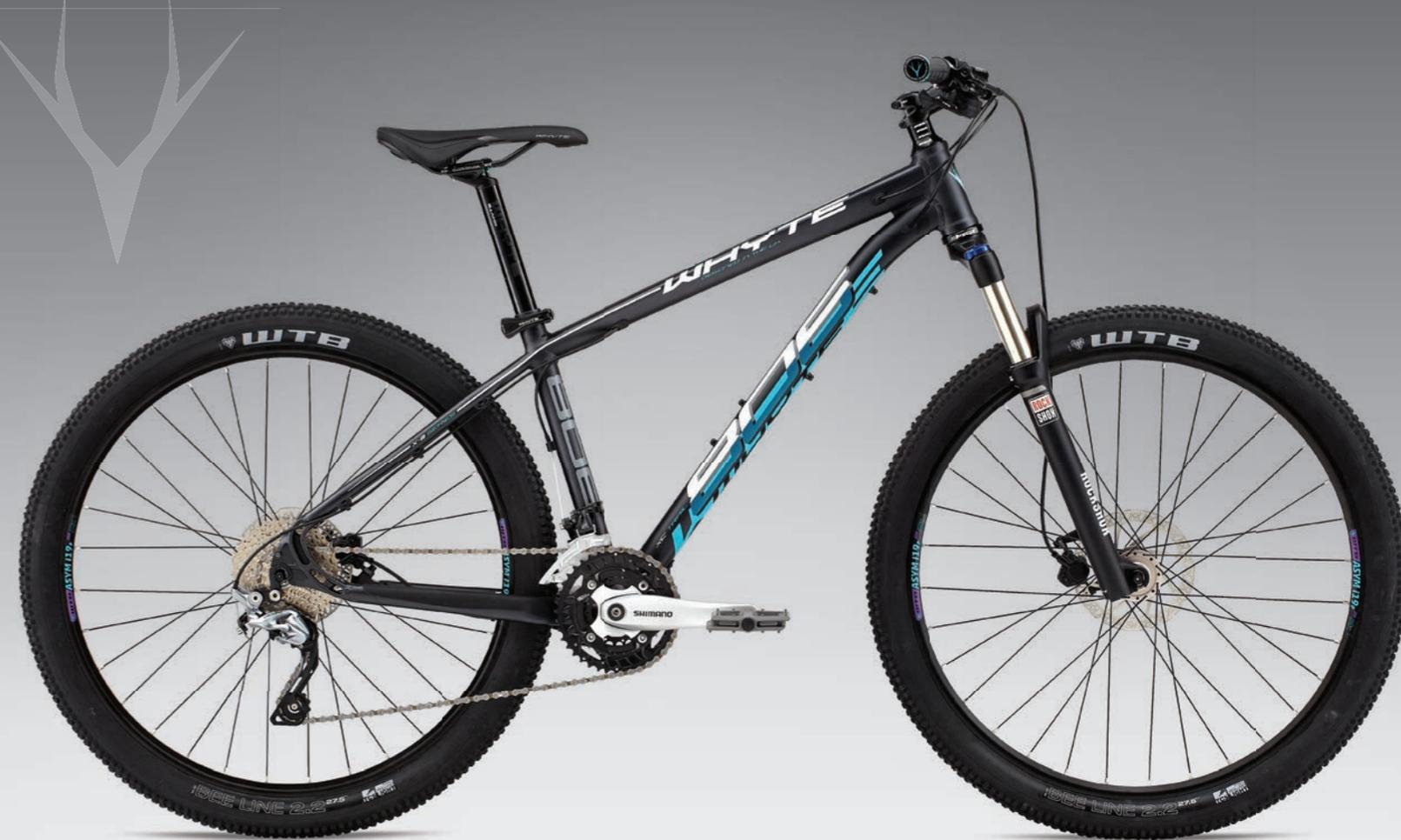
Shimano Deore 3x10spd drivetrain / Compact geometry and sizing down to XS for smaller riders / Adjustable air-sprung RockShox Recon Silver suspension fork
