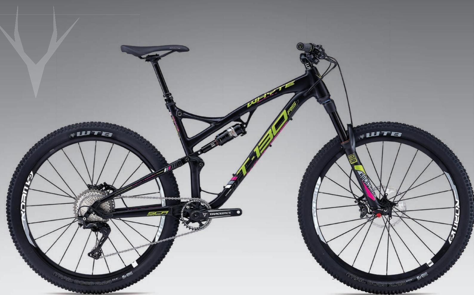
SCR frame with symmetrical chainstays for increased stiffness / Shimano XT 1 by 11 drivetrain / RockShox Pike fork, Monarch DebonAir shock and Reverb Stealth seatpost
