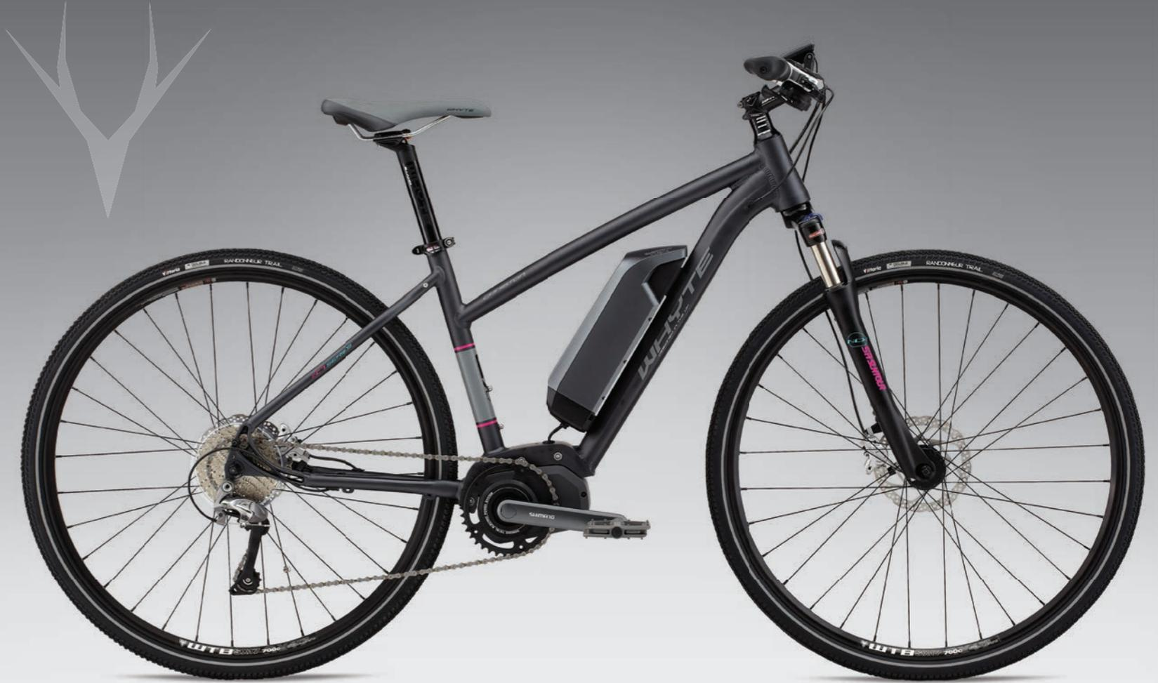
Wide-ratio 3x10spd Shimano Deore/LX gearing / Lightweight aluminium frame / Vittoria Randonneur Trail tyres with double puncture protection
